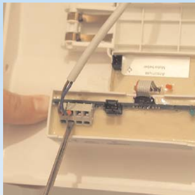
Connect 12V power supply
